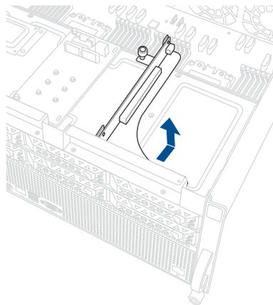
3. Place the riser card bracket on a flat and stable surface.
