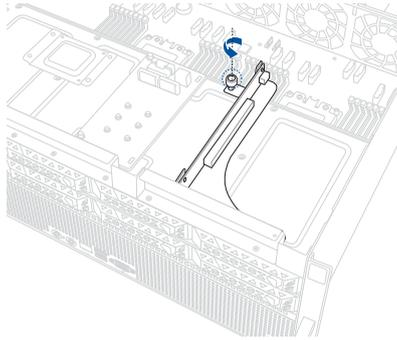
2. Firmly hold the riser card bracket, slide it towards the back of the chassis to unlock it, then pull it up to detach it from the chassis.
