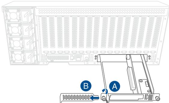
3. Insert and push the card all the way into the PCIe slot on the riser card (A), then flip the metal bracket lock back down to secure the card to the riser card bracket (B).
