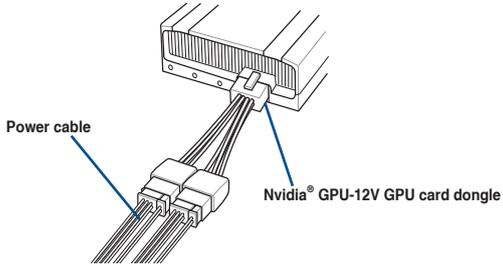
**Nvidia® GPU-12V or above GPU cards with ASUS GPU 8-pin power cable**
