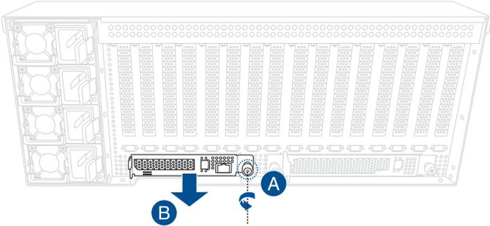
2. Flip the metal bracket lock open (A) then slide the metal bracket out of the left PCIe riser card bracket (B) and remove it.
