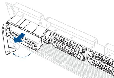
3. Prepare the 3.5" storage device then place the 3.5" storage device into the tray until it clicks into place.
