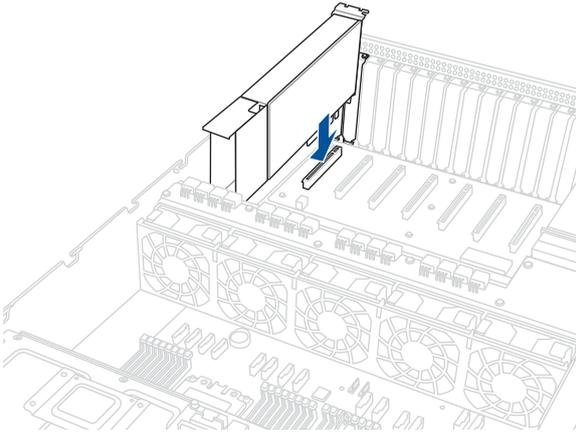
7. Attach the other end of the power cable (6-pin power connector) to an available 6-pin power connector on the middle of the server system, then secure the GPU card with the two (2) screws that you removed earlier in step 1.
