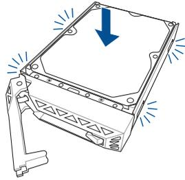
4. Push the drive tray and HDD assembly all the way into the depth of the bay until the tray lever and spring lock click and secure the drive tray in place.
