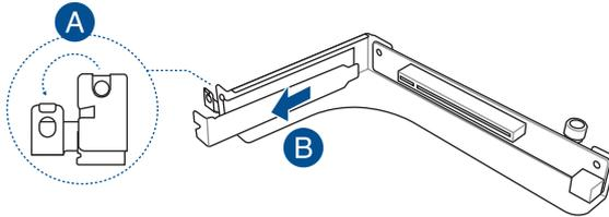
5. Insert the expansion card into the PCIe slot (A). Ensure that the golden fingers are totally inserted into the slot, then push the metal bracket lock clockwise until it locks and secures the expansion card to the riser card bracket (B).
