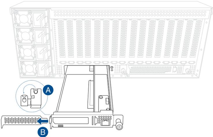
3. Prepare your expansion card and insert it into the PCIe x8 slot on the left PCIe riser card bracket.
