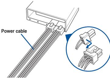
**Nvidia® GPU-12V or above GPU cards with power cable and Nvidia® GPU-12V GPU card dongle**
