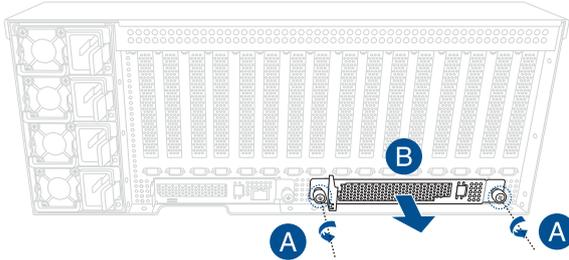
2. Flip the metal bracket lock up (A), and slide out the metal bracket (B).
