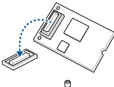
3. Push the PFR module down so that it is seated securely on the PFR module connector, then secure it using a screw.
