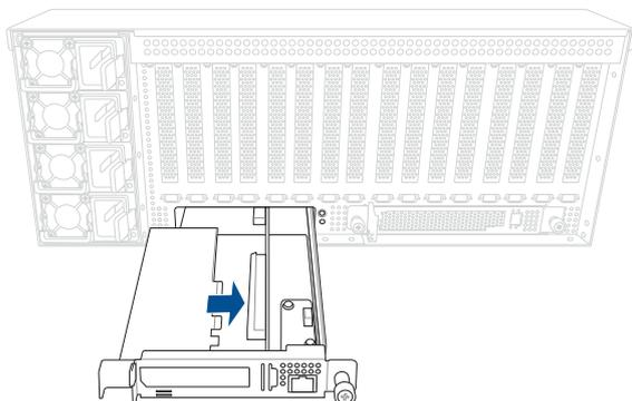
4. Once your expansion card is installed, flip the metal bracket lock back to secure the expansion card to the bracket.
