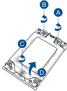
4. Slightly lift open the rail frame.
