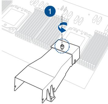
2. Lift the intake end of the air duct to remove it from the motherboard.
