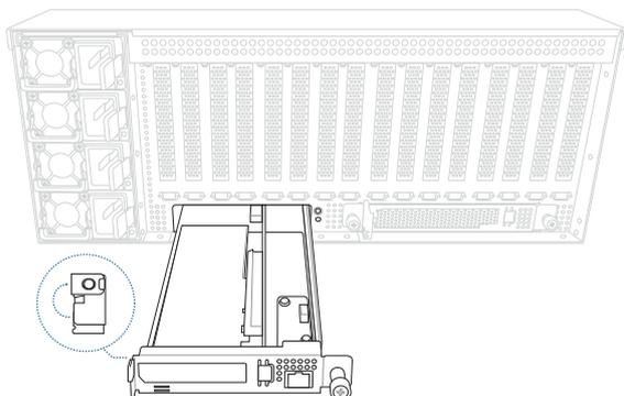
5. Push the riser card bracket back into the chassis until it is seated firmly in place (A), then secure it with the thumbscrews (B).
