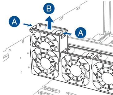
To reinstall the GPU fans, insert the fan into the fan cage. Ensure the fan connector is seated firmly within the cable holder.
