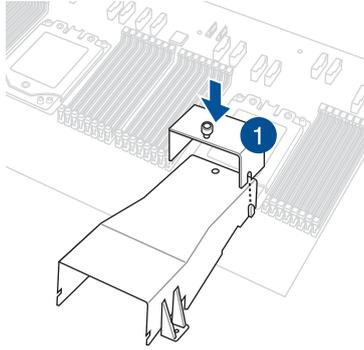
2. Secure the air duct to the motherboard by tightening the thumb screw.
