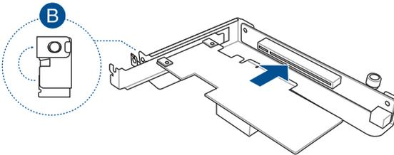
6. Align and insert the riser card and expansion card assembly into the chassis, then slide it towards the front of the chassis (A). Once in place, tighten the riser thumbscrew (B).
