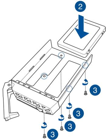
4. Follow step 4 of the **Installing a 3.5-inch storage device** section to replace the drive tray.
