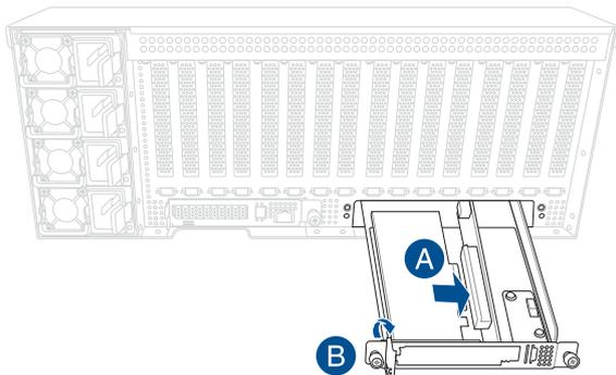
4. Push the riser card bracket back into the chassis until it is seated firmly in place (A), then secure it with the thumbscrews (B).
