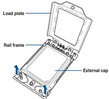
5. Slide the external cap out of the rail frame.
